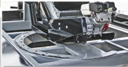
180° Swing with 9 individual indexing points for precise positioning of conveyor
