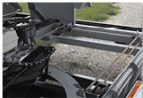
Shuttle allows for remote quick changes of seed boxes
