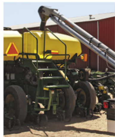
Telescoping tube can easily fill a central fill planter with one stop
