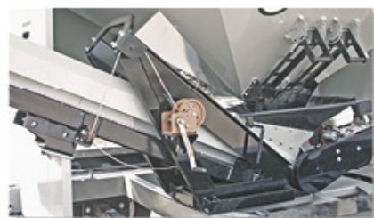
Discharge height adjusts with manual winch
