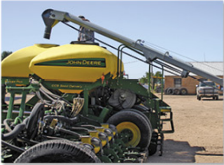
Optional telescoping belt conveyor extends from 14' to 22'*
