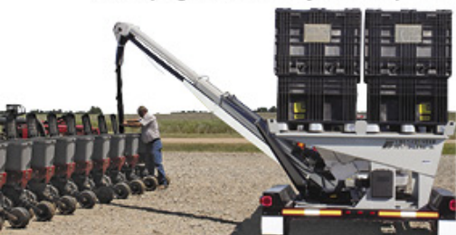
Telescoping belt can easily fill a 40' planter
